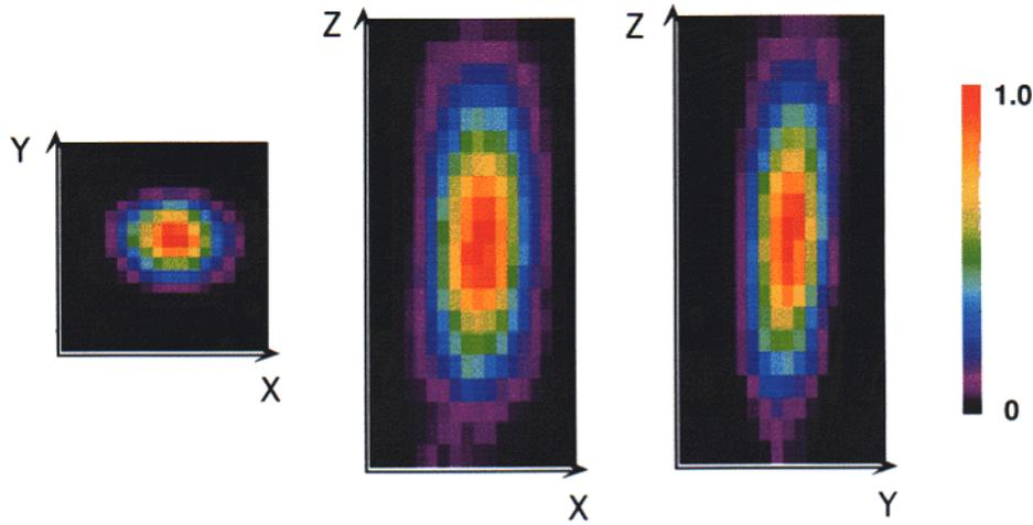
**Figure 4.** PSF of the two-photon set-up of figure 1; the PSF is obtained from the bead image with subsequent restoration with the bead object function. The pixels represent 40 nm in the lateral direction and 80 nm in the axial direction. The colour bar shows the normalized intensity values.
