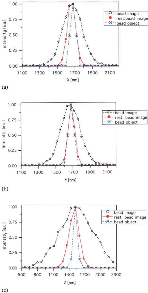
**Figure 3.** Profiles in X, Y and Z direction of the bead images, the restored data of the bead and the corresponding profile of an ideal spherical bead object.
