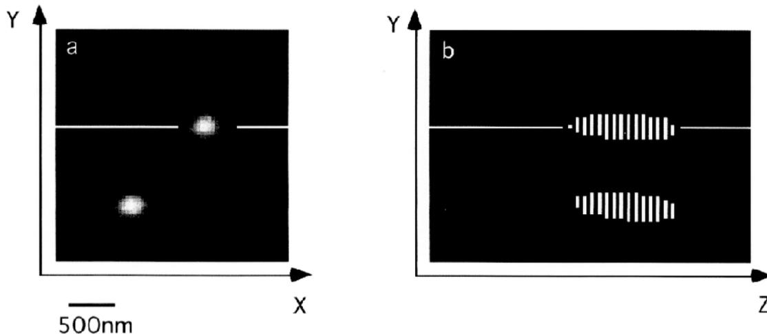
**Figure 2.** Two-photon image of two 120 nm fluorescence beads, (a) in XY, (b) projection of the data in Z at an intensity threshold of 25%.
