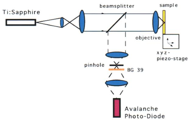
**Figure 1.** Set-up of the stage scanning two-photon excitation microscope. The fluorescence light passing an oversized pinhole is imaged onto the photosensitive area of an avalanche photodiode.
