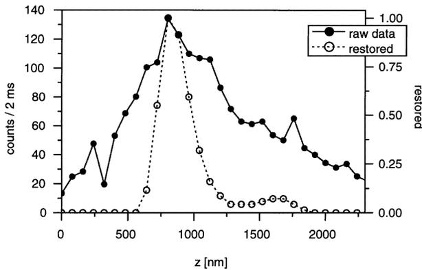
**Figure 10.** The actin fibre profile before and after restoration quantifies the three-fold increase of axial resolution in the fibroblast cell.
